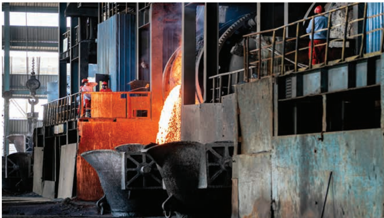
Copper production at CCS Isasmelt furnace
